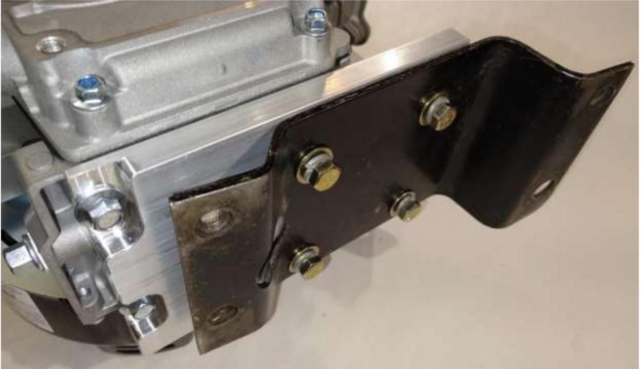
6. Set the engine into the Kitty Cat chassis and align the OEM plate to the bulkhead reinstalling original bolts finger tight.
